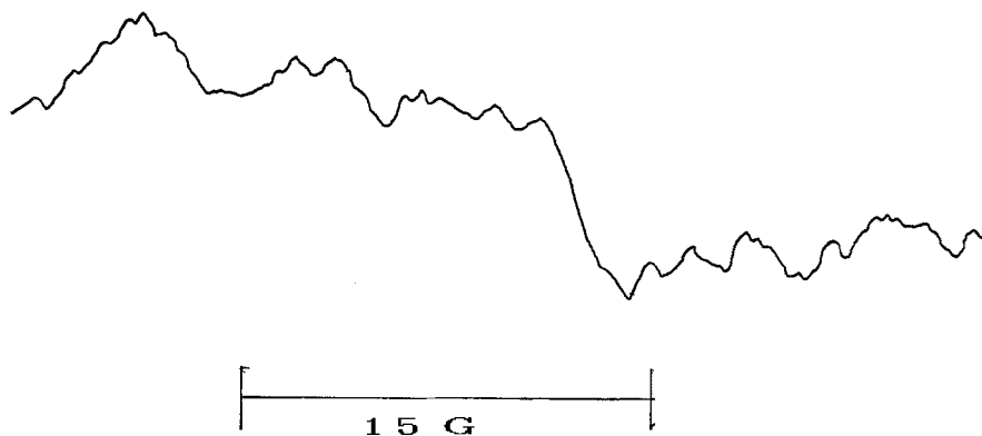
Fig. 5. ST + DPB + AIBN System. After 6 hours of heating at 78°C, and the spectrum was taken at 85°C. [DPB] = 0.30 M, [AIBN] = 0.03 M.
